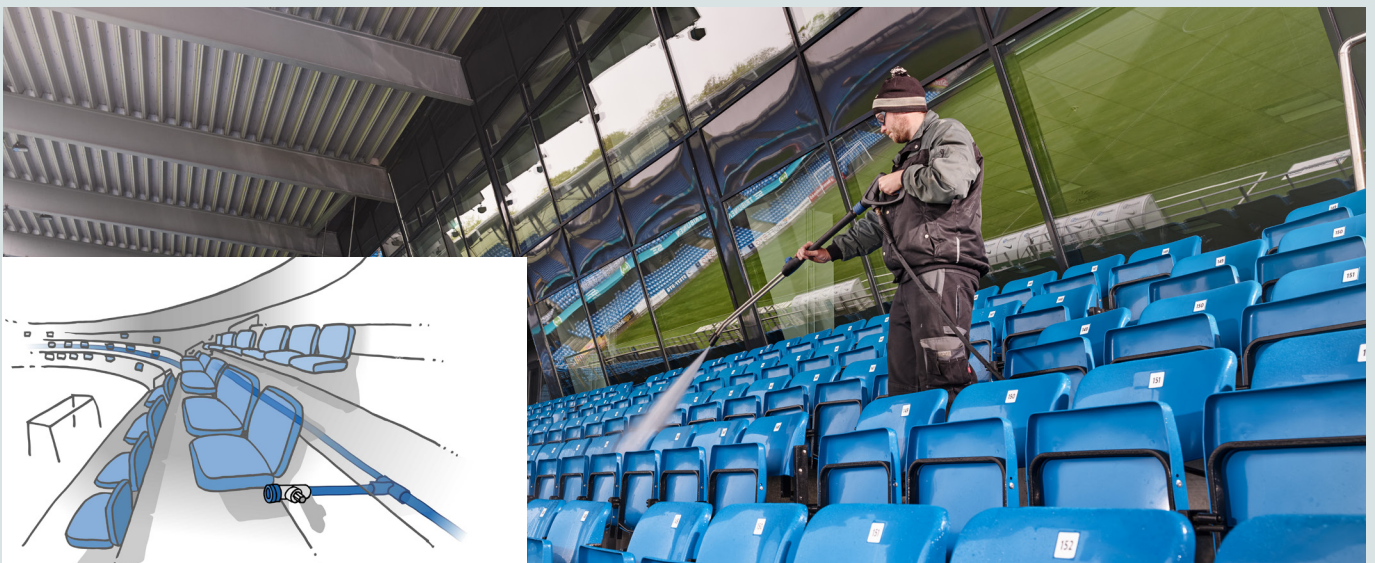
Cleaning of spectator area and seats in a stadium. Cleaning the spectator area after a game or an event can be difficult. In this example the stationary high pressure washer system (SC DELTA) enables multiple operators to clean fast and efficiently at the same time
