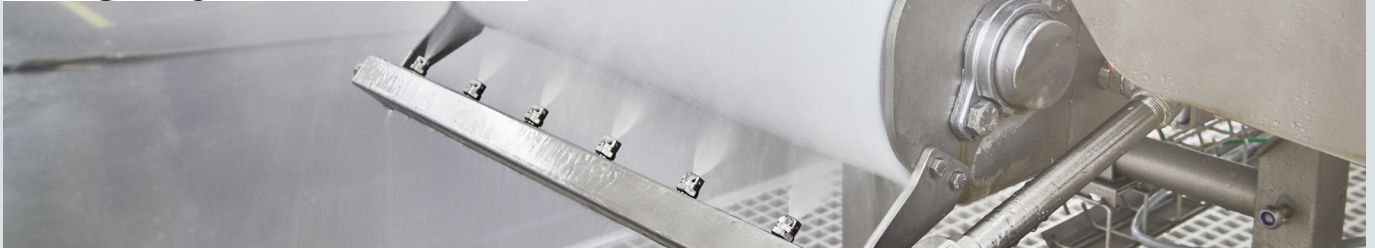
Conveyor belt cleaning in a large slaughter house. In this application the SC DELTA is fed with hot water needed together with high flow and pressure to achieve the desired result. SC DELTA enables several belts being cleaned at the same time
